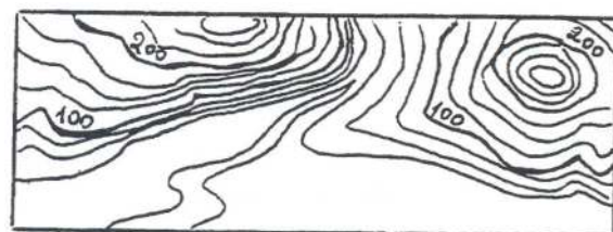
Figure 2 illustrates how contour lines illustrate the same location on a 2 dimensional map.
